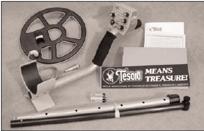
Assembly of the Vaquero is simple and requires no special tools. Just install the battery, mount the searchcoil on the lower pole assembly, connect the pole assemblies together, wrap the excess cable around the pole and, plug the cable into the control housing. Finally, adjust the pole length and searchcoil angle and you're ready!
