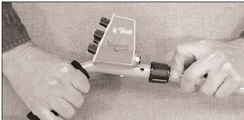
6. Slide the lower pole into the middle pole until spring buttons click into the first set of adjustment holes. Turn pole lock to tighten the assemblies into place.
