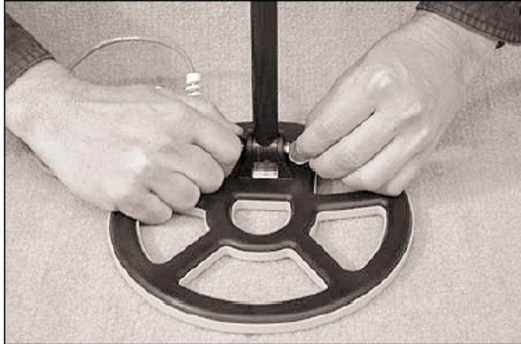
3. Insert the mounting screw through the holes in the mounting ears and pole tip—entering from the side opposite the cable connection.
